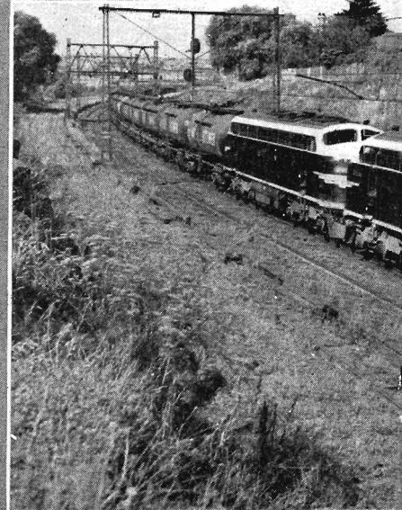
BULK BITUMEN: Eight special 70-ton capacity Adelaide freight train for the transport of this type of consignment. The train was hauled
