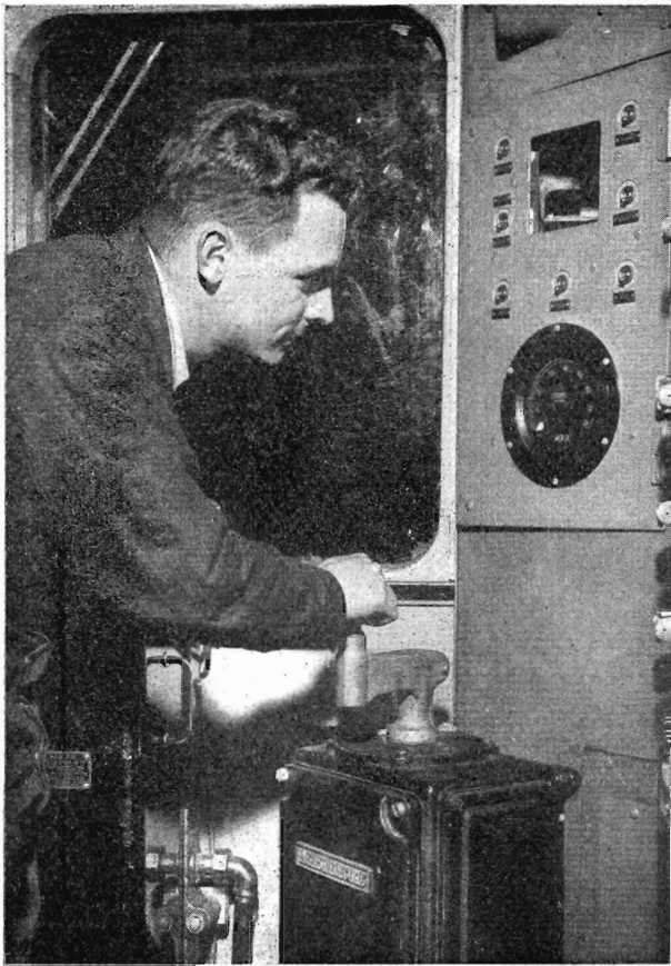
In sequence tests, the various controllers and switches are worked to make sure that they and associated equipment are functioning correctly.
