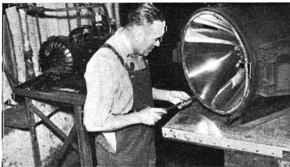
Repairs to a locomotive headlight. The generators for the lights (one is shown in the background) run at the high speed of 3,600 revolutions a minute. With their powerful 600-foot beams these headlights play an important part in railway safety.
