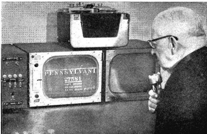
Yard manager demonstrates use of TV on Richmond, Fredericksburg and Potomac Railroad in recording wagon numbers of incoming train.
